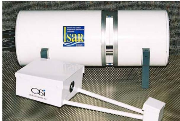
**Figure 2-5:** External view of the ISAR showing the shutter open. The optical rain sensor is in front
