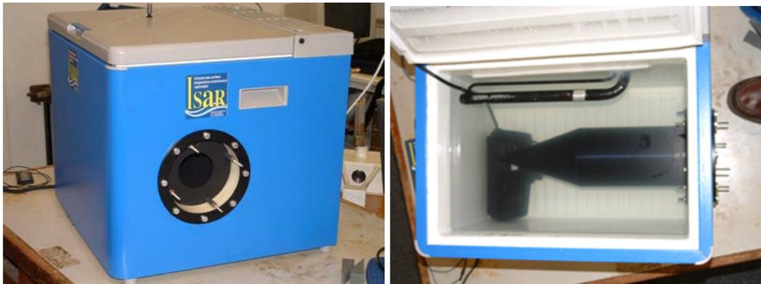
**Figure 2-8.** The CASOTS-2 Black Body used as the laboratory reference for calibrating or validating the ISAR before and after each ship deployment. **Left:** External view showing the black body cavity aperture and blanking plates. **Right:** Internal view of the water bath revealing the conical end of the cavity. The black object to the left is the pump for stirring.
