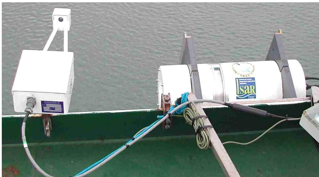
**Figure 2-6** The ISAR and rain detector mounted on the *Pride of Bilbao*.
